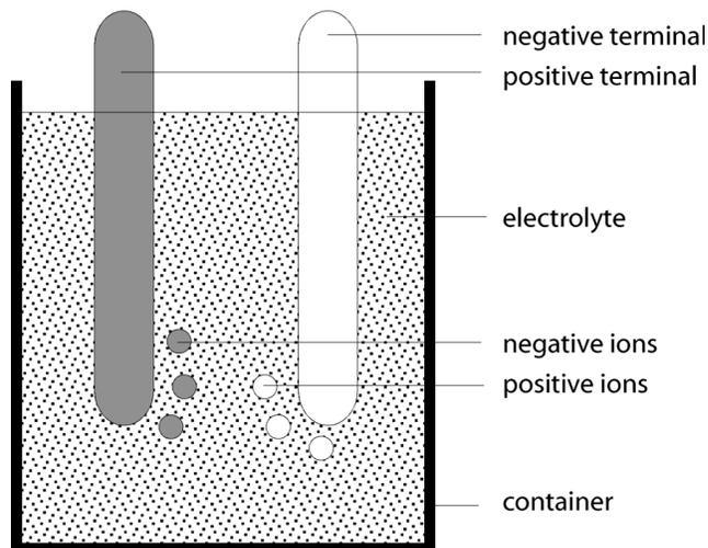
Reactions at both posts quickly stop. The negatively charged zinc post pulls back any positive ions that try to enter the electrolyte; the positive carbon post pulls back any negative ions that try to enter the electrolyte. This is why a battery in storage can last for long periods of time.
