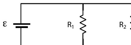
**CONFIGURATION** • One battery, two equal light bulbs—side by side (in *parallel*).
