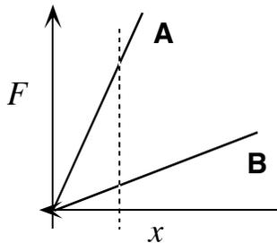
To get the same stretch, indicated by the vertical dotted line, more force must be applied to spring A.
