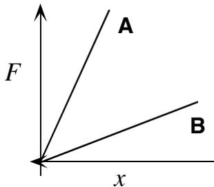
Two springs, A and B were tested here. The slope of A's graph is greater than that of B's graph.
