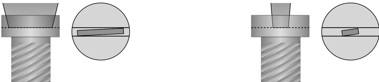
5. Which—if either—screwdriver would be more effective in loosening a screw: one with a blade as wide as the screw's groove or one with a blade wider than the screw's groove? Explain.
