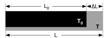
The black rectangle indicates the size of the bar at the low temperature  $T_0$ . The gray region shows the expansion that occurs upon warming to T. This growth is greatly exaggerated in the diagram. If the bar were cooled back down to  $T_0$ , its size would return to that indicated in black.
