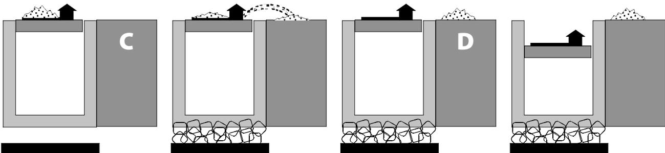
**CD.** Once the piston reaches the high elevation, the heat is turned off. As grain is pitched off the elevator, the gas is cooled. During this process, the pressure is reduced to its original value.
