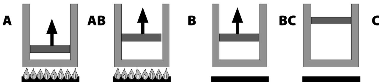
**AB.** As the story begins, the piston is rising. It had a "head start," in the sense that it was already moving up before we saw it. But 6545 J of heat are added nonetheless to keep it motivated. Since the gas is expanding upward faster than the added heat would force it to, the pressure is dropping. It drops to half its original value while the volume doubles. The temperature remains constant.
