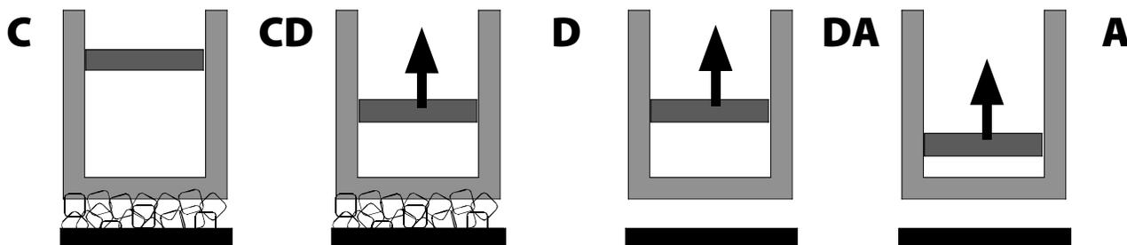
**CD.** Heat is removed. The gas contracts to half its previous volume. The pressure increases to double its previous value. The temperature remains constant.
