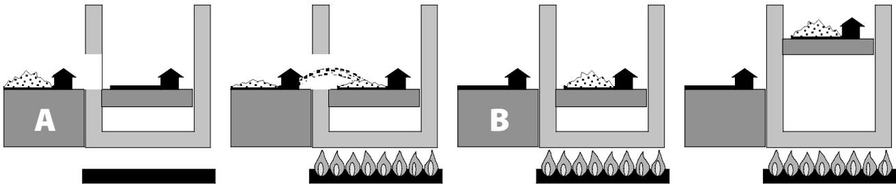
**AB.** As grain is pitched onto the elevator, heat is added to the gas. The elevator does not move up, but the pressure quadruples.
