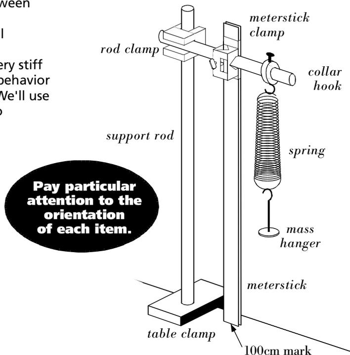
2. Load Force. This is the weight of the slotted masses. Convert the slotted mass values to kilograms and multiply that mass by gravitational acceleration to determine the weight of the load.
