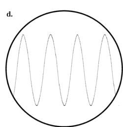
Which is which? The diagrams above indicate oscilloscope traces for sounds. (Sound is a *longitudinal* wave. When sound waves hit the diaphragm of the microphone, the diaphragm is set into oscillation. This oscillation is transformed into an electric signal. How? Good question. Ask your teacher! Anyway, the oscilloscope, in effect, displays the sound wave—but as a *transverse* wave. The oscilloscope crests correspond to sound wave compressions; the troughs correspond to expansions.)
