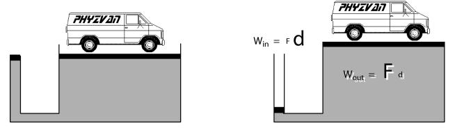
A big force is needed to lift the auto. A person exerts a small force over a large distance via the small piston on the left to produce a large force lifting the auto. The force acting on the auto, however, acts over a small distance.
