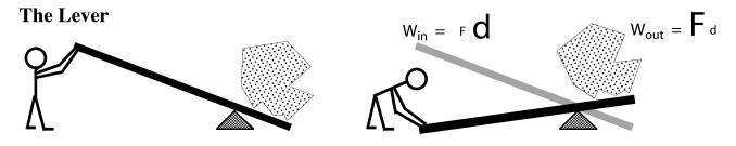
A big force is needed to lift the rock. The person exerts a small force over a large distance to produce a large force acting on the rock. The force acting on the rock, however, acts over a small distance.
