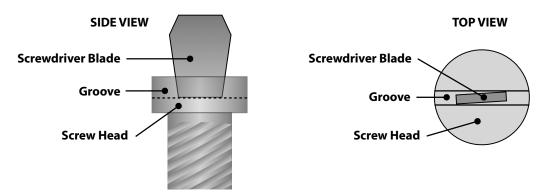
4. Which screwdriver will be more effective in loosening the stubborn screw: the one with a wide blade or the one with a narrow blade? Explain.
