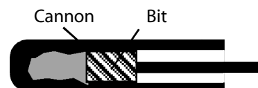
The brass cannon is spun around a fixed bit. A sharp blade scrapes off MORE material than a dull blade, yet generates LESS heat in the process.
