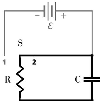
2. Which statement best characterizes the current when an uncharged capacitor is being charged?
